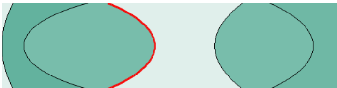
Figure 25. Cross section of two lens pairs with the default color table “White and Mint”. Air is marked light green. Glasses are marked by different shades of dark green. The third surface is currently selected and thus marked red.
