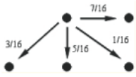
Figure 155. Weighting factors for distribution of quantization errors to neighboring positions during Floyd-Steinberg quantization.
