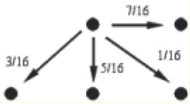
Figure 789. Weighting factors for distribution of quantization errors to neighboring positions during Floyd-Steinberg quantization.
