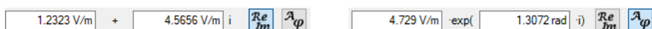
Figure 10. Example of a control to enter a complex value with physical units.
