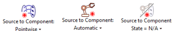
Figure 351. The different states of the ribbon buttons to analyze the settings for propagation from source to components. The propagation between components and to detector follow the same logic.
