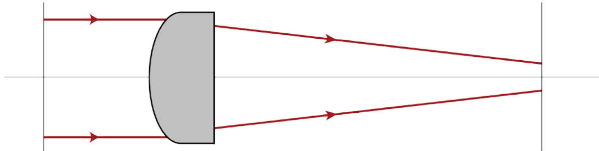
Convex-Planar lens Radius of First Interface: R Center Thickness: d
